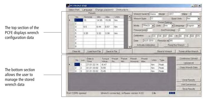
The right upper half of the PCFE window displays data such as tool serial number, make, model, torque span and units of measurement. The date of calibration and the period of calibration are also shown in this section.
