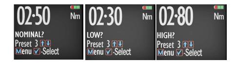
Step 9: Once the parameters have been confirmed the operator can find the task within Preset Mode. Use to select Preset Mode from the main menu to find the task.
