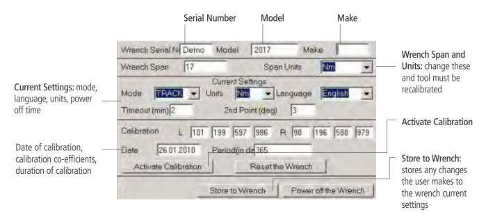
The left upper section displays the presets stored in the tool - the user can choose to use the PCFE to set the presets or it can be done manually on the tool.
