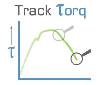
As torque is applied, the driver will actively display the applied torque reading from 5% up to the max span of the device. On removal of the torque load the display will return to zero.
