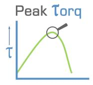
In Peak Mode, on condition that the torque loaded is above 10% of the tool span, then the maximum torque reading will remain displayed when the torque load is removed. The user has the option to store the reading in memory. If storage of the reading is not required, the user may continue to the next measuring task.
