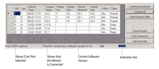
Each row will display the following: time and date of torque operation, torque value and units. If it's a preset result then the minimum and maximum tolerances are displayed along with the nominal setting
